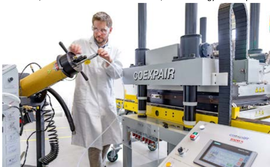
Figure 10 Composite door manufacturing at Coexpair
