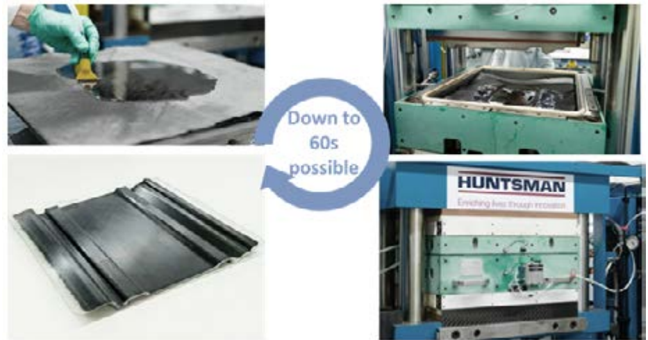
Figure 3 Schematic representation of the Dynamic Fluid Compression Moulding (DFCM) process
