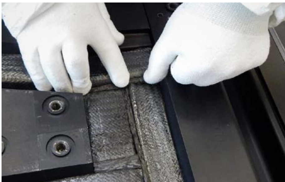
Figure 9 RTM composite process: the injection and cure of the full structure is done in only one operation
